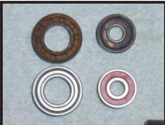
Top: The old bearings from the Saito FA-65 Bottom: New bearings for the .65 from Saito.
