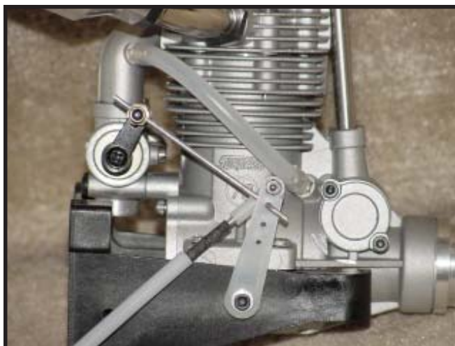
The Dubro linkage applied to my OS 70 Super II. Note the Sullivan Precision Rod connected to a ball link on the backside of the bellcrank.
